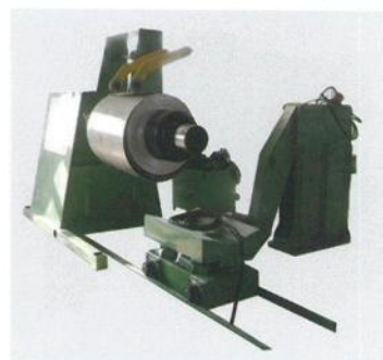
▶ 悬臂、液压自动式放料架 Cantilever hydraulic automatic De-coiler
