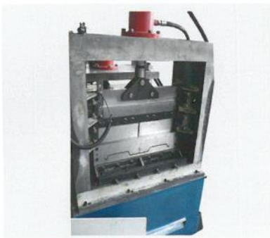
▶ 液压切断 Hydraulic cutting with waste
