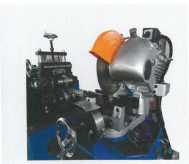
▶ 无毛刺锯切 Circular saw cutting
