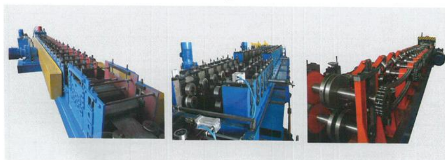
▶ 墙板式机架+链条传动 Wall Frame+Chain Driven
