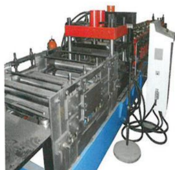
▶ 5辊校平机带送料带冲切 Five Rollers Leveler with punching&cutting
