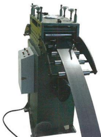
▶ 9 辊校平机 Seven Rollers Leveler
