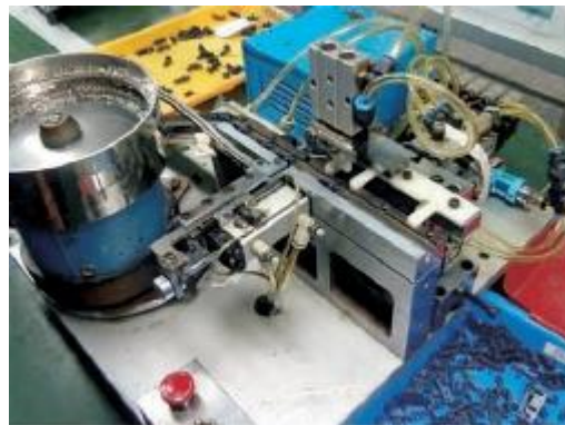
压螺母治具 Nut pressing fixture
