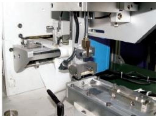
贴标治具 Marking fixture
