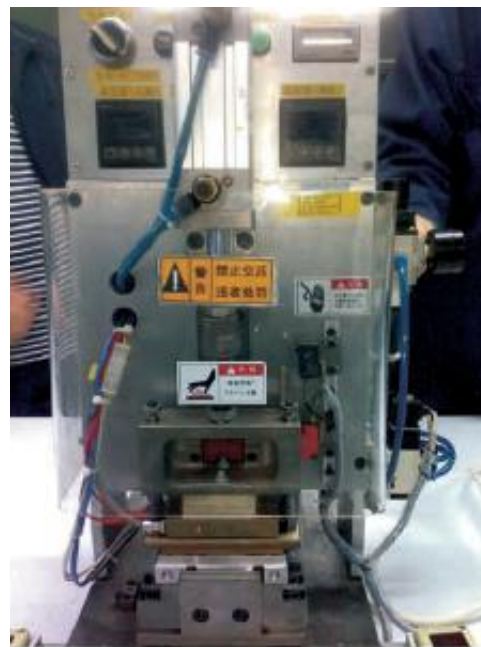
电阻焊治具 Resistance welding fixture
