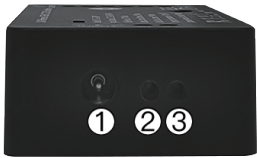
① 5.5x2.1mm DC Socket ② ③ V+,V- power interface
