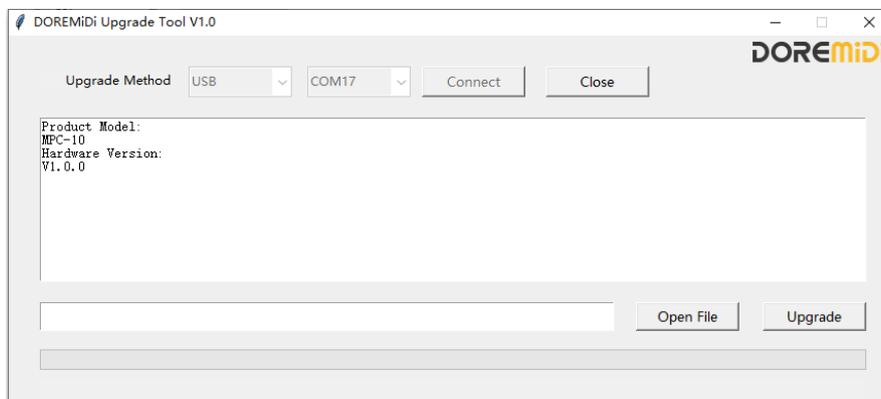
**Step 3:** Click "Open File", select the upgraded firmware MPC-10\_Vxxx, click "Upgrade", and wait for the upgrade to be completed "Upgrade completed!".
