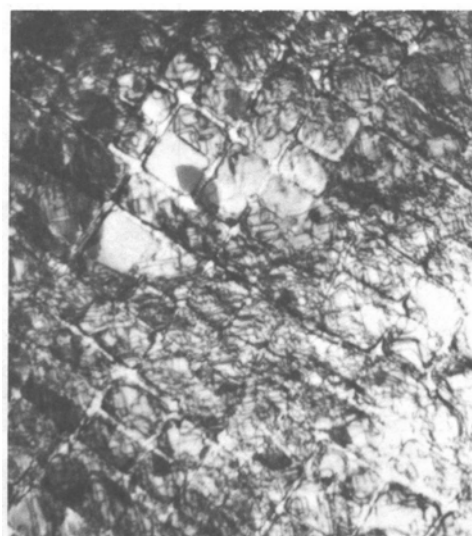
Fig. 18 Homogeneous deformation in CMSX-2 ( T_2 heat treatment) after 0.16% creep strain at 760 °C (1400 °F). Source: Ref 29
