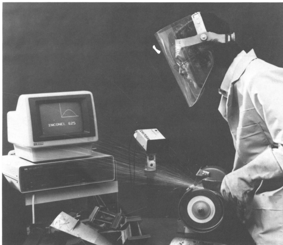
Fig. 6 Identification of scrap by experimental spark analysis equipment
