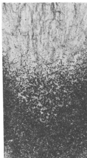
Fig. 1 Fracture surface of as-cast chilled iron. White, mottled, and gray portions are shown at full size, top to bottom.
