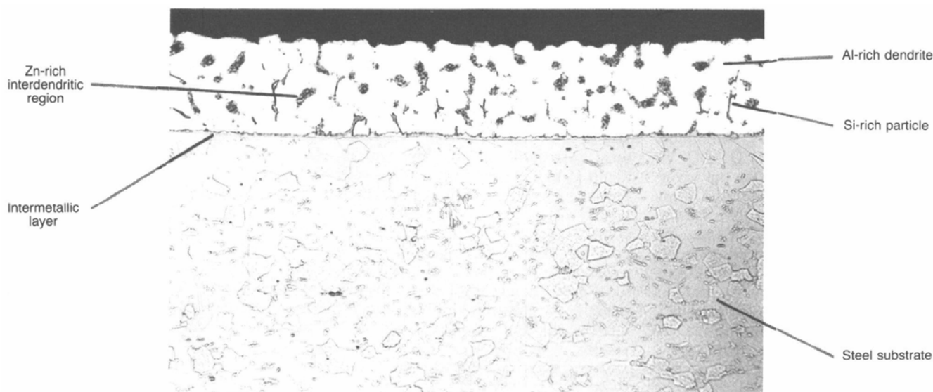
Fig. 9 Microstructure of an aluminum-zinc coated sheet. Etched with Amyl nital. 500×
