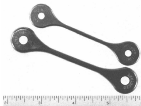
Fig. 23 Tensile bars specially developed for testing MIM. Courtesy of Omark Industries, Advanced Forming Technology, and Metal Injection Molding Association
