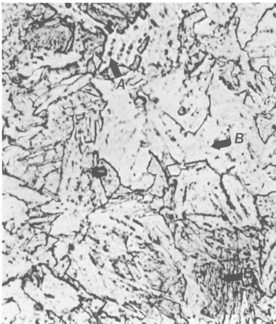
Fig. 6 Heat-affected zone exhibiting a wide variety of microstructures in the intercritical and subcritical regions. A, spheroidized carbides; B, bainite and martensite
