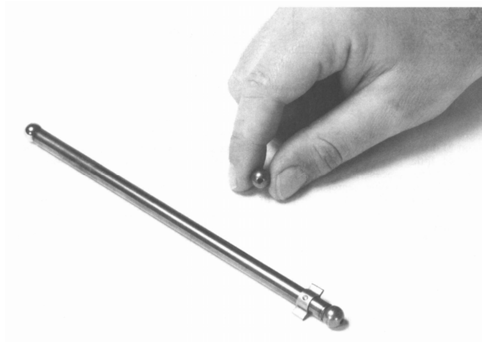
Fig. 23 Automotive push-rod assembly with wear-resistant spherical CPM 10V tips. Courtesy of Crucible Materials Corporation
