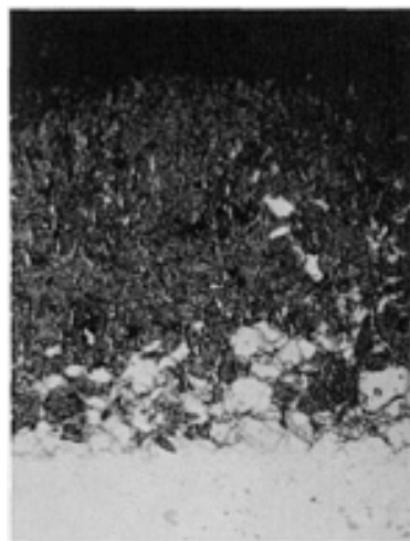
Fig. 8 Observable diffusion zone on the unetched (white) portion of an ion-nitrided 416 stainless steel. Nital etched. 500×
