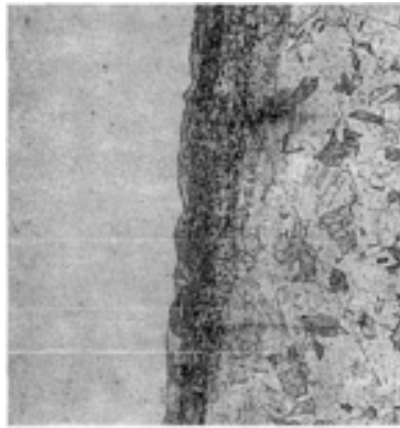
Fig. 4 Etching of 70-30 brass reveals smeared layer
