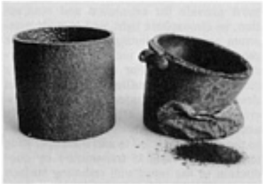
Fig. 14 Comparison of high-temperature (1350 °C, or 2460 °F) creep testing of radiant tube sections. (a) Silicon-silicon carbide composite after 360 h. (b) Ni-Cr-Fe alloy after <1 h
