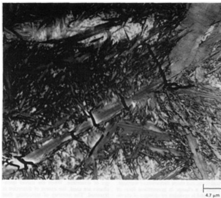
Fig. 13 Microcracking in a Ni-Cr steel. Source: Ref 67
