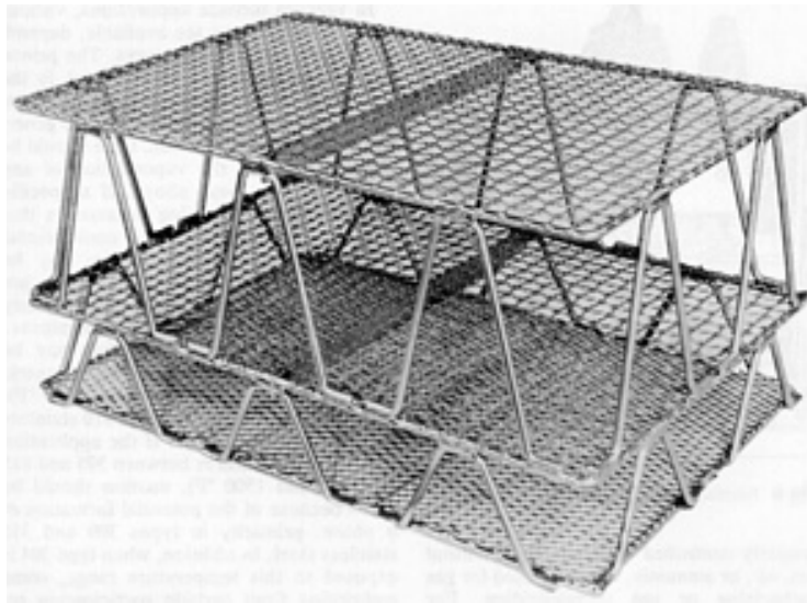
Fig. 8 Fixture designed for heat treating shafts
