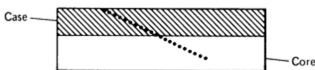
Fig. 4 Cross-sectioned specimen for hardness-traverse method of measuring depth of light and medium cases. Dots show locations of hardness-indenter impressions.
