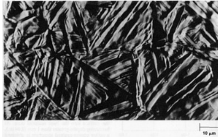
Fig. 15 Surface relief of a normalized C 45 steel sample polished before hardening that had the isothermal energy transfer at approximately the melting temperature. Energy density transferred, 1250\text{ J} \cdot \text{cm}^{-2} ; surface roughness, R_z , is 1.2\text{ }\mu\text{m} ( 48\text{ }\mu\text{in.} ). Source: Ref 9
