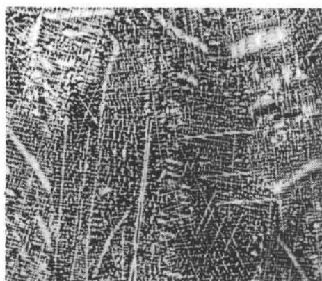
Fig. 31 Copper alloy C71500 (copper nickel, 30%) ingot. Dendritic structure shows coring: light areas are nickel rich; dark areas are low in nickel. 20x. Source: 85ASM
