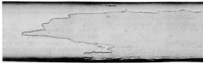
Fig. 24 Recrystallized microstructure of doped tungsten wire
