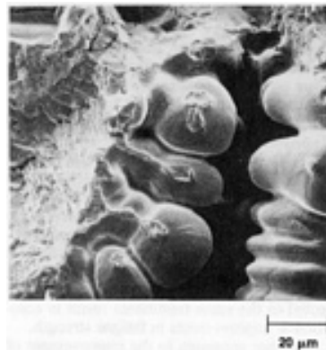
Fig. 6 Dendritic structure present in the surface shrinkage porosity of an as-cast Ti-6Al-4V component
