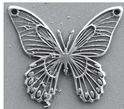
A micro-butterfly, printed by del Pozo. The width is around 70 micrometers. Courtesy of Eindhoven University of Technology.
