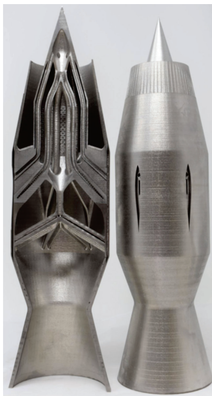
Fig. 5 — Cut view of a test ramjet engine, additively manufactured with laser powder bed fusion (L-PBF) using Haynes 282 superalloy, a material that can survive the temperature extremes of hypersonic flight.
