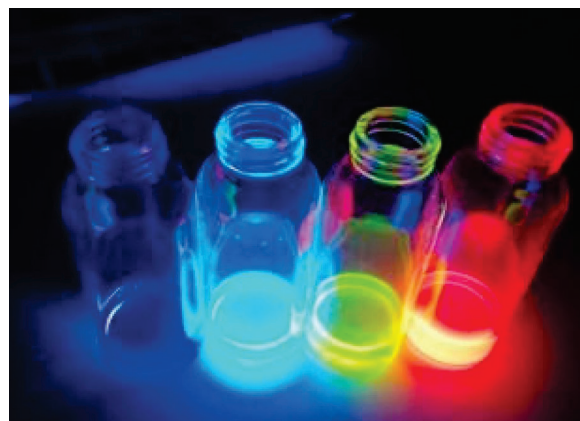
Nanomaterials of perovskite dispersed in hexane and irradiated by a laser. Courtesy of Luiz Gustavo Bonato.
