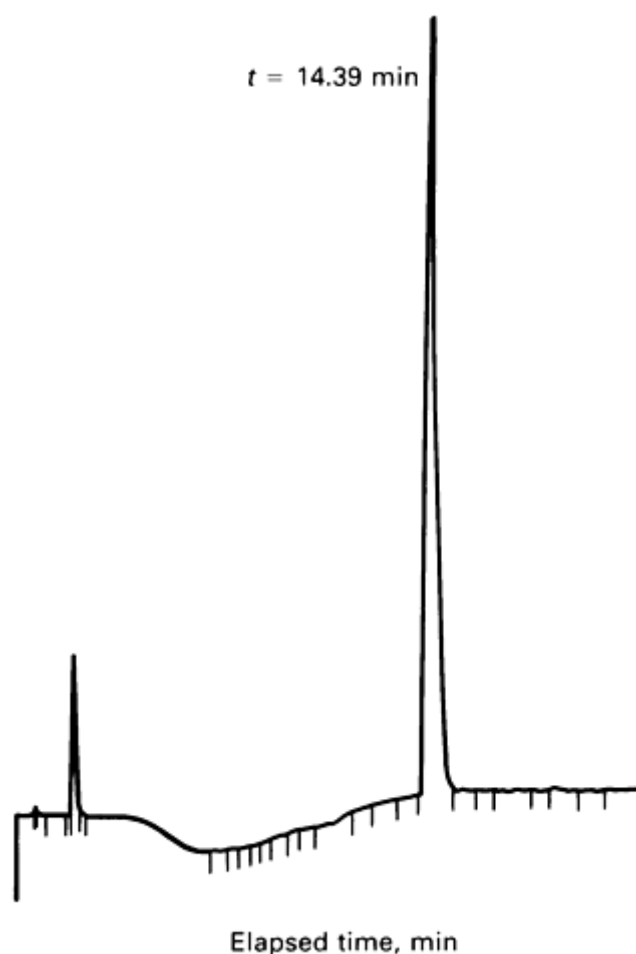
Fig. 13 Reversed-phase chromatogram of the product of the first step in the synthesis shown in Fig. 12.
