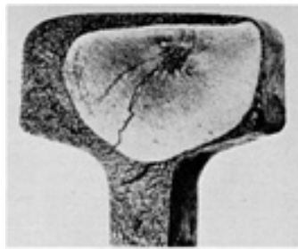
Fig. 11 Transverse fracture of an AISI 1075 steel railroad rail. Fracture nucleus (dark area near top of railhead) initiated a fatigue crack (large light area around nucleus).
