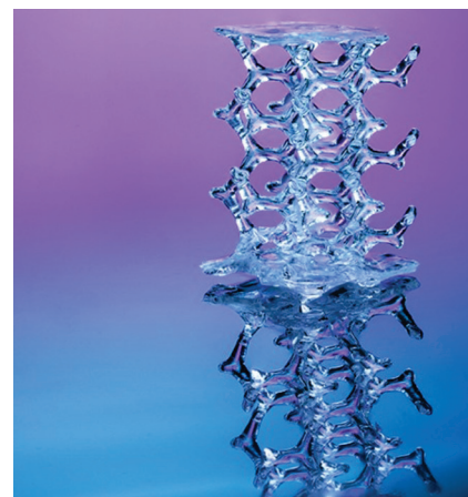
Microscopic object made of silica glass using volumetric additive manufacturing.
