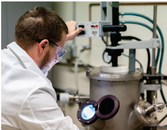
Doctoral student William Trehern operating a vacuum arc melter—a synthesis method commonly used to create high-purity alloys of various compositions. Courtesy of Texas A&M Engineering.
