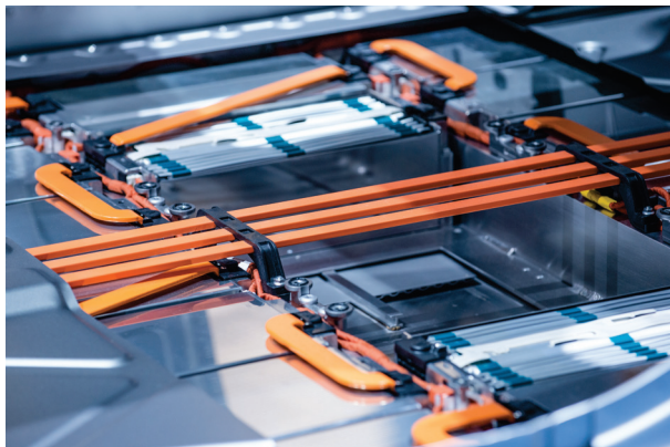
Electric car lithium battery pack and power connections.
