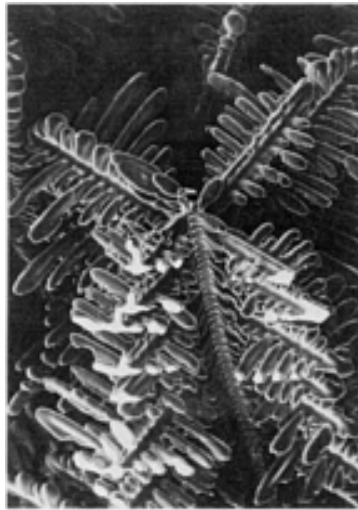
Fig. 8 Directionally solidified peritectic cobalt-samarium-copper alloy showing primary cobalt dendrites when the \text{Co}_{17}\text{Sm}_2 matrix is etched away. The cut surfaces in the foreground indicate the structure that would be observed on the plane of polish if the matrix were not etched away.
