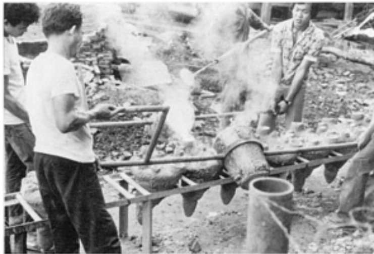
Fig. 14 Contemporary casting of bronze into lost wax investments in Thailand.
