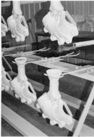
Fig. 2 Completed EPS pattern assemblies ready for ceramic coating. Courtesy of R.E. Grote, Missouri Precision Castings
