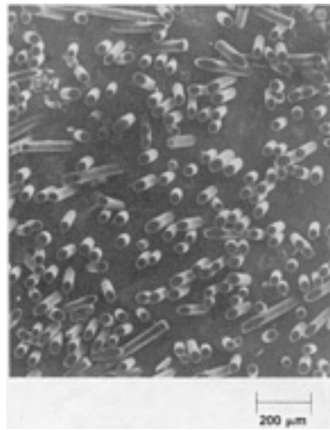
Fig. 8 SEM micrograph of electrochemically etched vertical section of cast Al-4Mg/23 vol% alumina fiber composite showing random planar orientation of fibers. Courtesy of R. Mehrabian.
