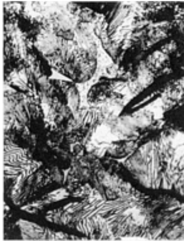
Fig. 9 Steadite in gray cast iron. Etched using 2% nital. 400×. Source: Ref 12
