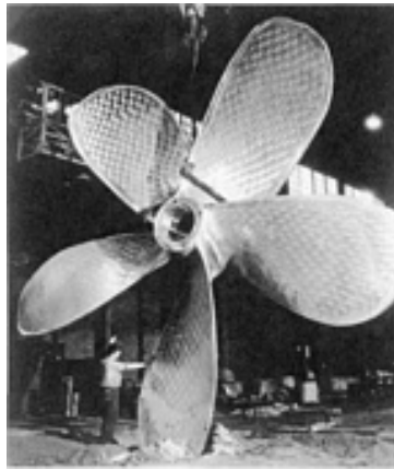
Fig. 26 Propeller for a 114,000 ton tanker measures 7.5 m (24.7 ft) in diameter and weighs 37.52 Mg (82,725 lb). Part was machined and polished from a single 53.75 Mg (118,500 lb) nickel-aluminum bronze casting. Courtesy of Baldwin-Lima-Hamilton Corporation.
