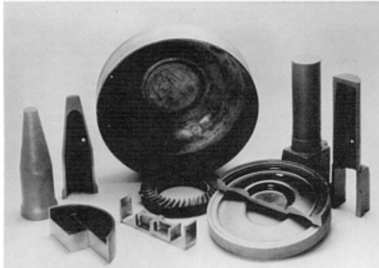
Fig. 3 Typical ferrous and nonferrous parts produced by squeeze casting. Dome in center measures 423 mm (16.5 in.) in outside diameter and weighs 29.5 kg (65 lb). Courtesy of IIT Research Institute
