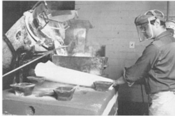
Fig. 3 Pouring of a sand mold for a magnesium-zirconium alloy casting using the fluxless technique. Courtesy of Haley Industries Ltd.
