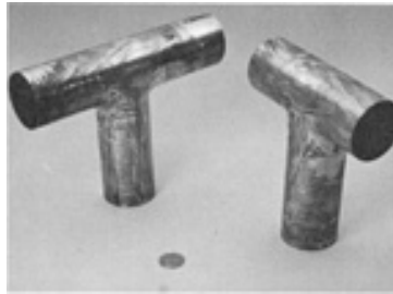
Fig. 19 Magnesium/graphite fiber tubes produced by filament winding and vacuum casting. Courtesy of Martin-Marietta Company.
