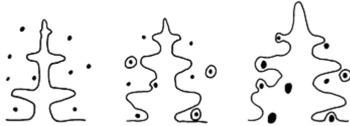
Fig. 20 Schematic illustrating the progression of growth in austenite-SG eutectic.
