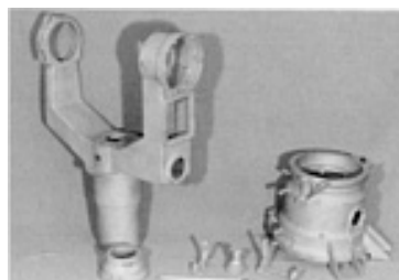
Fig. 15 Titanium housings for military optical applications produced by the investment casting process.
