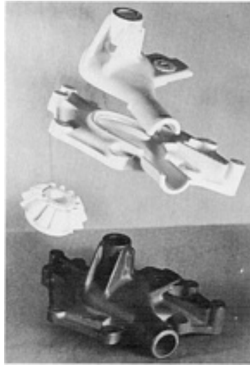
Fig. 3 Expandable polystyrene pattern and finished casting produced by lost foam casting
