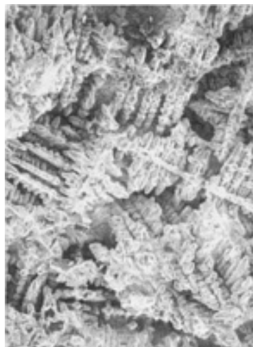
Fig. 19 SEM view of shrinkage cavities in heavy-section gray iron. 20×
