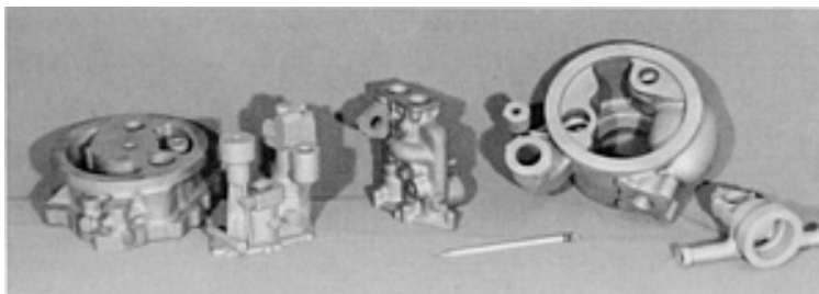
Fig. 14 Titanium hydraulic housings produced by the investment casting process.
