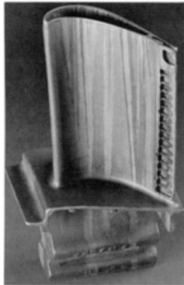
Fig. 1 Directionally solidified thin-wall turbine blade cast from Alloy CM 247 LC (modified MAR M-247 composition)
