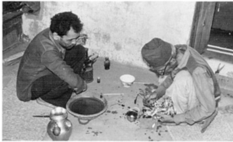
Fig. 11 Amalgam gilding in Patan, Nepal. The work, including heating of the amalgam to sublime the mercury, takes place in the open air on the roof of the workshop.
