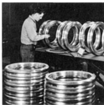
Fig. 25 Centrifugally cast aluminum bronze worm gear blanks being inspected. Courtesy of Wisconsin Centrifugal, Inc.
