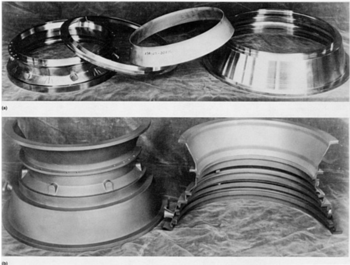
Fig. 10 IN718 turbine casing for a helicopter engine that was originally produced from four forgings and spinnings (a). The assembly was replaced by a hot isostatically pressed casting, which is shown in cross section in (b). Courtesy of General Electric Company
