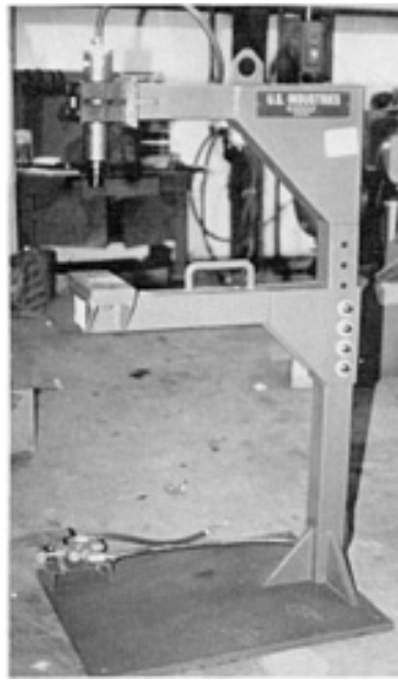
Fig. 3 Vertical core knockout machine. Courtesy of United States Industries
