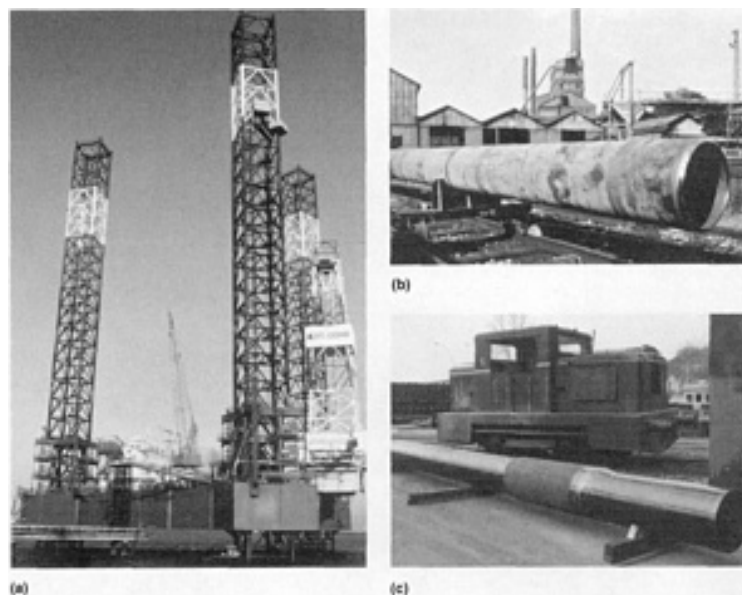
Fig. 6 Offshore petroleum production applications for centrifugally cast parts. (a) Jackup leg. (b) Risers. (c) Buckle-crack arrestor.
