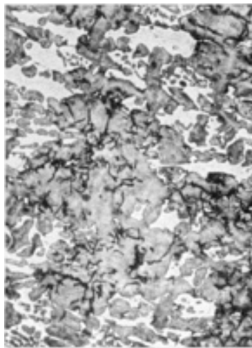
Fig. 8 Mottled cast iron etched using 4% picral. The white phase is eutectic carbide. 50×. Source: Ref 10
