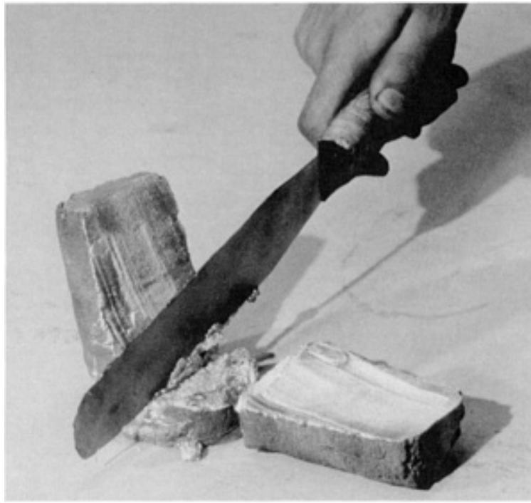
Fig. 2 Semisolid aluminum billet being cut by a spatula
