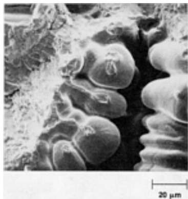
Fig. 4 Dendritic structures present in the surface morphology of an as-cast titanium component.
