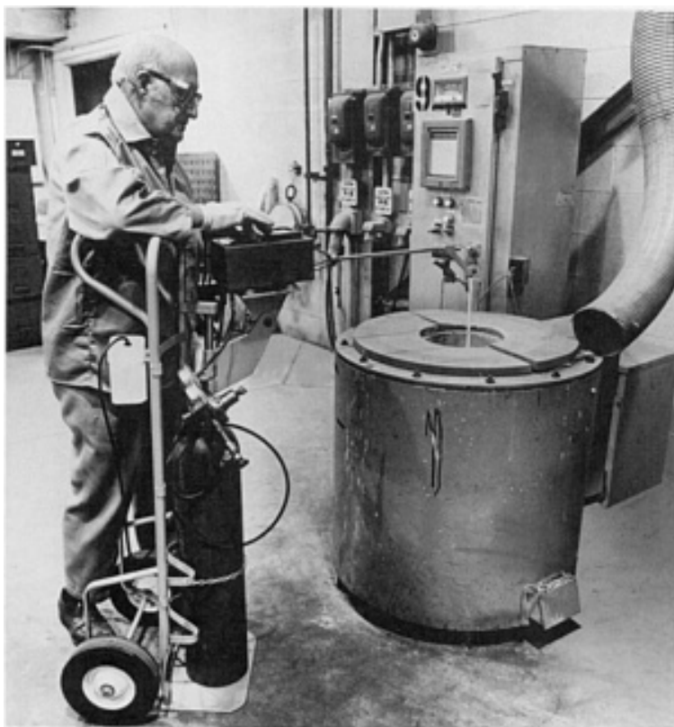
Fig. 21 The Telegas unit for hydrogen determination. Courtesy of Aluminum Company of America.
