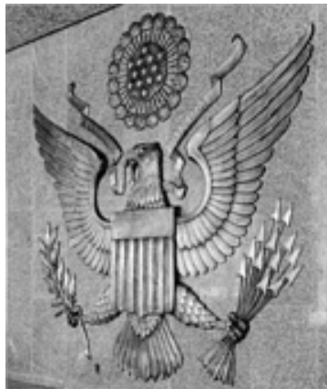
Fig. 28 Twelve foot high bronze sand casting of the Great Seal of the United States located in lobby of the Federal Deposit Insurance Corporation building in Washington, D.C. Weight, 1.8 Mg (4000 lb).
