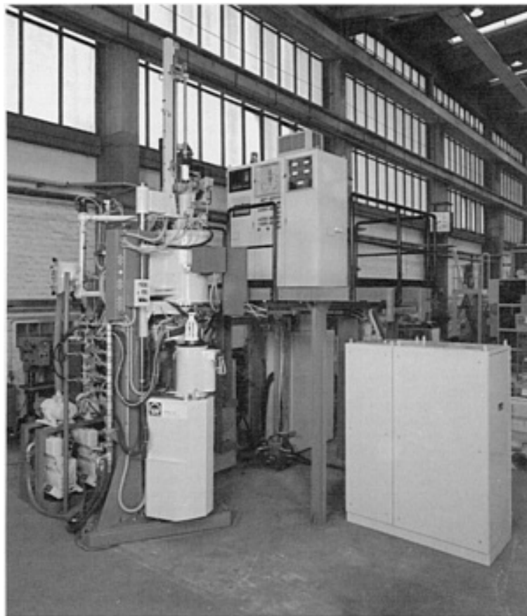
Fig. 13 Computer-controlled vacuum precision casting furnace showing the mold chamber.
