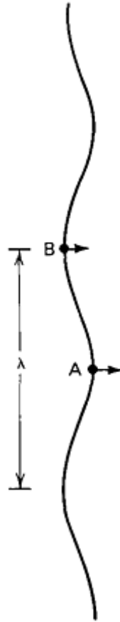
Fig. 5 Perturbed shape of the interface with wavelength \lambda . The linear stability analysis determines the condition when the velocity of point A is less than that of point B.
