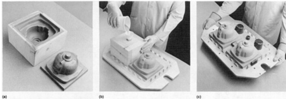
Fig. 3 Steps in producing a match plate pattern from a master pattern. (a) Wood master pattern is constructed with appropriate shrinkage factors included. A reverse from the master pattern. (b) Reverse mold is used to cast the polyurethane pattern on the aluminum match plate. (c) Reverse mold is removed, and a wood gating system is added. Gating can also be cast on with the pattern or made from aluminum stock. Courtesy of W. Allen, Allen Pattern of Michigan
