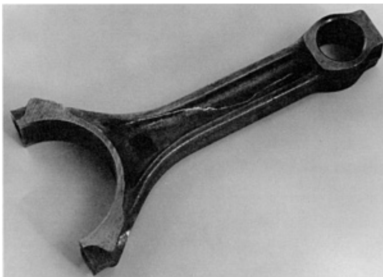
Fig. 27 Black light used to reveal magnetic particle indication of a lap that could lead to potential failure of a forged connecting rod. Courtesy of Magnaflux Corporation
