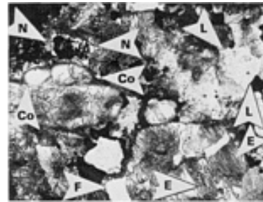
Fig. 89 Same as Fig. 87, but etched. Arrows N show nickel-rich region, inside which are martensite platelets. The effect of the 1% Cu is indicated by shading or coring of the ferrite (arrows Co). Arrows E show eutectoid; arrows L, an underetched region of eutectoid. Arrow F indicates a white ferrite grain. 2% nital. 310×
