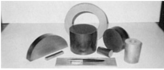
Fig. 2 Examples of monolithic blocks of sintered P/M materials used to machine prototype parts. Courtesy of Powder-Tech Associates
