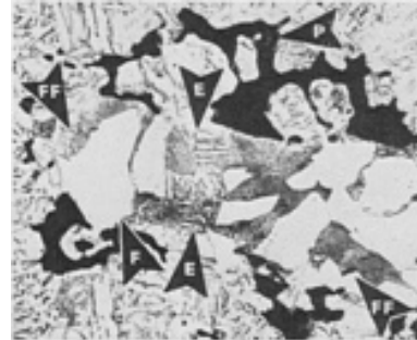
Fig. 79 Prealloyed steel (Fe-1.85Ni-0.6Mo-0.5C, 6.7 g/cm 3 ), with an impurity particle of unalloyed free ferrite (outlined by arrows FF), which has a carbon content of 0.3 to 0.4%. It is a mixture of proeutectoid ferrite (arrow F) and normal eutectoid (arrows E). Compare this eutectoid with the matrix eutectoid. Arrow P indicates a pore. 2% nital. 365×
