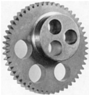
Fig. 4 Eccentric gear for a washing machine made of iron alloy powder containing 2% copper and 0.5% graphite. Center hole inside diameter: approximately 19 mm (0.76 in.); eccentric outside diameter: approximately 57 mm (2.28 in.); total thickness: approximately 28.50 mm (1.14 in.); eccentric thickness: approximately 15.90 mm (0.63 in.); pitch diameter: approximately 115 mm (4.59 in.)
