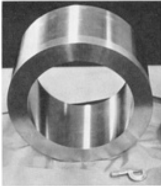
Fig. 11 Silver-infiltrated tungsten billet for rocket nozzle throat liner. Source: Ref 42
