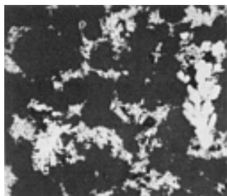
Fig. 4 Electrolytic copper powder, showing dendritic structure. 85×
