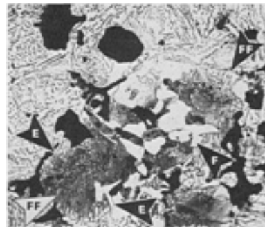
Fig. 80 Same as Fig. 79, with a similar unalloyed iron particle. Arrows FF outline the free ferrite, which has a carbon content of approximately 0.6%, judging by its pearlite (arrows E) and its white proeutectoid ferrite (arrow F). 2% nital. 365×
