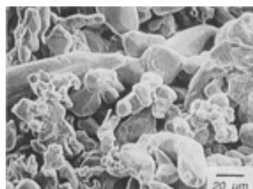
Fig. 1 Sponge fines made by the Hunter process
