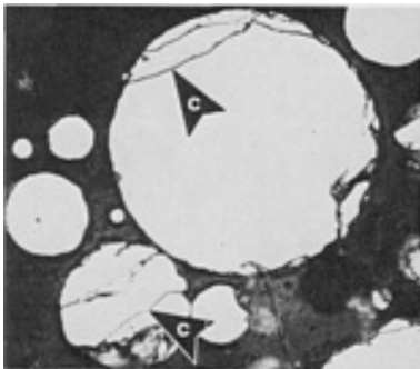
Fig. 159 Fe-31Si, water-atomized master-alloy powder (-100 mesh). Regular particle shape implies low green strength. Particles cracked (arrows C) during processing. As-polished. 645×
