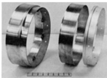
Fig. 20 Aluminum alloy engine inlet mounting assembly for an aircraft before (right) and after (left) assembly by electromagnetic forming. Courtesy of Grumman Aircraft Systems
