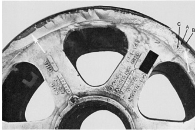
Fig. 1196 Portion of an aircraft landing wheel of sand-cast magnesium alloy AZ81A-T4, showing a corrosion-fatigue fracture that occurred in service at the locking-ring channel. Nominal tensile strength was 276 MPa (40 ksi). The fracture extended halfway around the perimeter of the wheel. Many discolored, crescent-shaped fatigue-crack nuclei were found; two are indicated by white arrows. See Fig. 1197, 1198, 1199, and 1200 for TEM views of areas at A, B, and C. 0.3x
