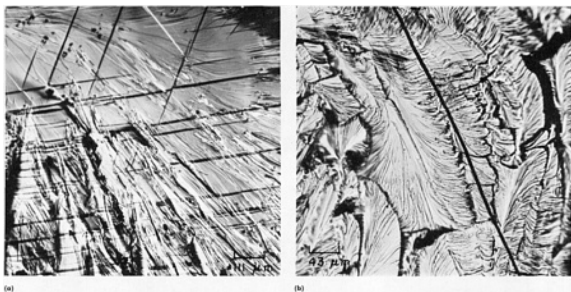
Fig. 5 Cleavage fractures in room-temperature impact specimens examined by C.A. Zapffe. (a) Cast polycrystalline antimony (99.83Sb-0.04S-0.035As-0.035Pb-0.015Fe-0.01Cu) (b) Vacuum-arc-cast high oxygen
