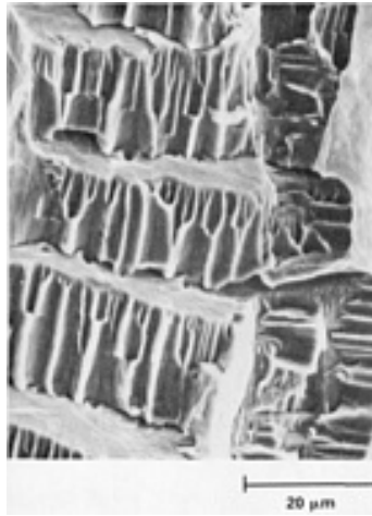
Fig. 39 Flutes and cleavage from SCC of \beta -annealed Ti-8Al-1Mo-1V in methanol. Source: Ref 89
