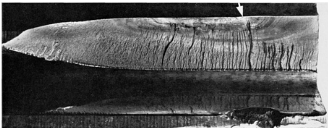
Fig. 246 Surface of a fatigue fracture (similar to that in Fig. 245) that occurred, after 841 h of service, in a tooth of the right-side bull gear of the same tractor. This gear also was made of AISI 1053 steel and induction hardened. Hardness of this gear was similar to that of the gear in Fig. 245 except that the depths at which hardness was 50 HRC were 12.2 mm (0.48 in.) below the tip of the tooth and 9.5 mm (0.37 in.) below the surface of the root fillet. The arrow indicates the fatigue-crack origin. The damage to the tooth just below the one that fractured probably resulted from jamming by a fragment from the fracture. \sim 2.5\times
