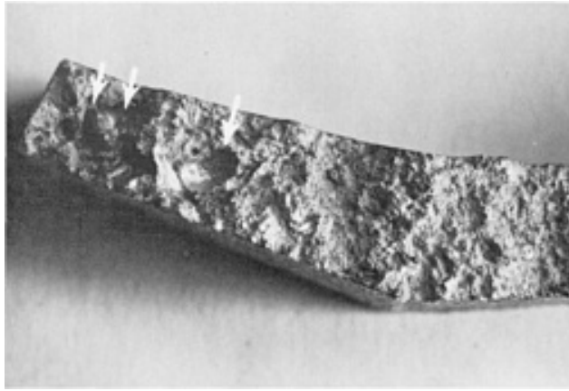
Fig. 923 This fracture surface is from the bracketed edge of the sand-cast carrier tray in Fig. 921. Like the surface shown in Fig. 922, the one here exhibits the characteristics of brittle fracture, there being no sign of a shear lip at any of these edges. Again, there is evidence of porosity; the arrows point to quite large gas cavities. The cavities could have been caused by a reaction between the liquid metal and organic binders in the sand mold, or could have resulted from entrapped air being carried into the mold by undue turbulence in pouring the casting. 3×
