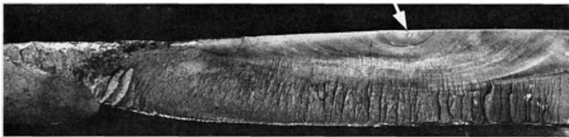
Fig. 245 Surface of a fatigue fracture that occurred, after 732 h of service, in a tooth of the induction-hardened AISI 1053 steel left-side bull gear of a tractor. Hardness of the tooth was 57 HRC at the tip and 50 HRC at a depth of 13.3 mm (0.52 in.). Hardness in the root fillet was approximately 56 HRC near the surface and 50 HRC at a depth of 11.5 mm (0.45 in.). The arrow indicates the origin of the fatigue crack. See also Fig. 246, 247, and 248. \sim 2.5\times
