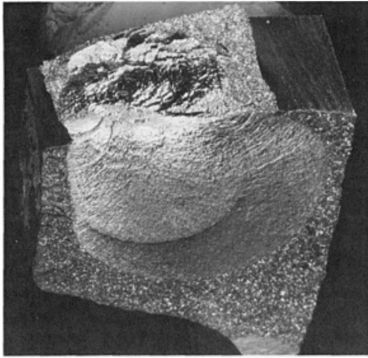
Fig. 69 Macrograph of broken rail showing the interconnection between the shell fracture (across the top) and the detail fracture (on the transverse plane). 3.5 \times . (R. Rungta, Battelle Columbus Laboratories)
