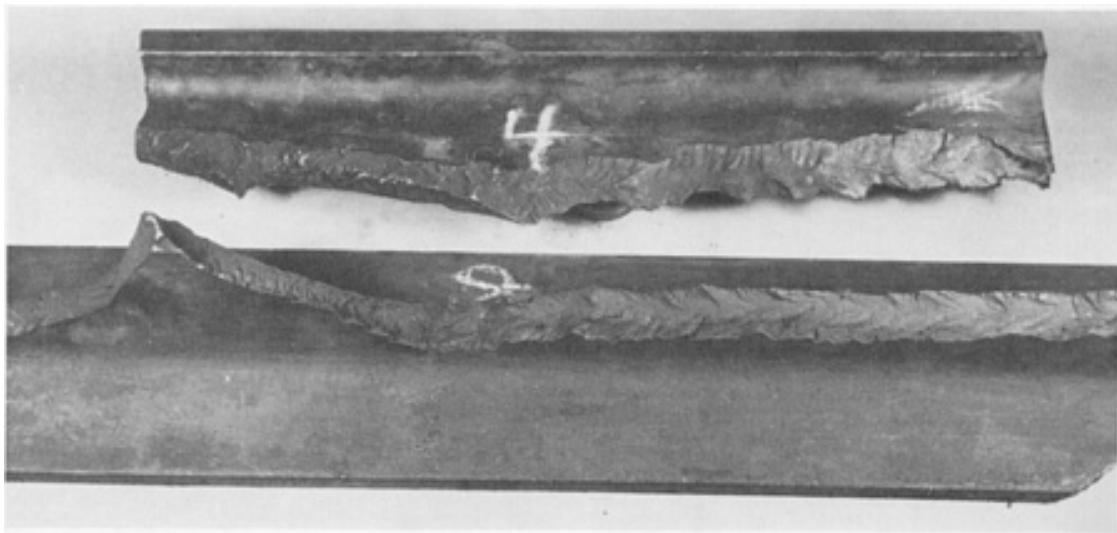
Fig. 39 Classic appearance of chevrons on a brittle fracture of a steel railroad rail. The fracture origin is not on the section shown.
