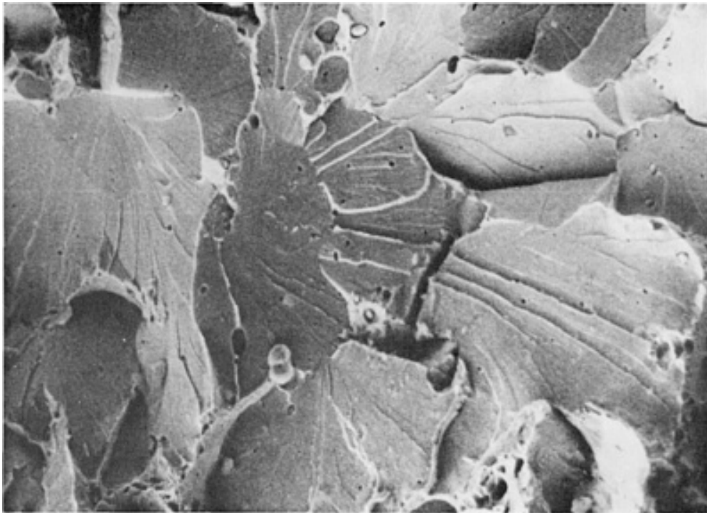
Fig. 119 Brittle fracture of AISI 1020 hydraulic jack shaft. Failure originated at root of machined thread. Corrosion (evident on part) and fatigue (due to repeated loading of shaft) may also have played roles in the failure. Photomicrograph of fracture surface shows transgranular cleavage with individual grains identified by changes in fracture plane orientation. The apparent grain size of 100 to 125 \mu\text{m} corresponds to a ductile-to-brittle transition temperature of approximately 100 °C (212 °F). SEM, 450× (J.M. Rigsbee, University of Illinois)
