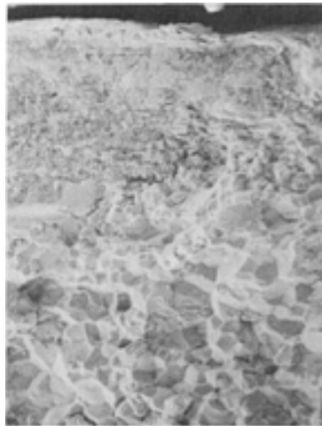
Fig. 540 Brittle intergranular fracture of AISI 9254 due to quench cracking. The crack initiated at a seam, 0.15 mm (0.006 in.) deep. The seam wall is the irregularly textured area at top in the fractograph. SEM, 200 \times (J.H. Maker, Associated Spring, Barnes Group Inc.)
