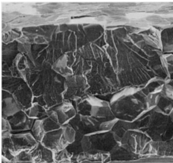
Fig. 1090 The external surface (top) and the corrosion-fatigue fracture surface (bottom) of a solution-treated and peak-aged Al-5.6Zn-1.9Mg sample tested in deaerated 0.5 mol NaCl at a cathodic potential of -1.6 V (SCE). Compare with Fig. 1089, 1093, and 1095. SEM, 100 \times (R.E. Ricker, University of Notre Dame, and D.J. Duquette, Rensselaer Polytechnic Institute)
