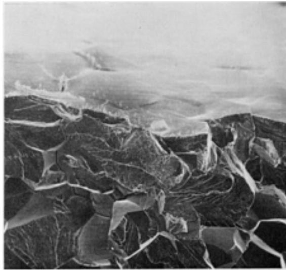
Fig. 1089 The external surface (top) and the corrosion-fatigue fracture surface (bottom) of a solution-treated and peak-aged Al-5.6Zn-1.9Mg sample tested in high-purity deaerated water. SEM, 100 \times (R.E. Ricker, University of Notre Dame, and D.J. Duquette, Rensselaer Polytechnic Institute)
