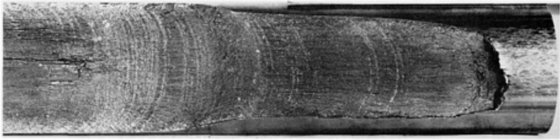
Fig. 205 Fatigue-fracture surface of the shaft of a forging hammer of AISI 1144 steel containing 0.45% C, 1.60% Mn, and 0.28% S. The fatigue crack began at a heavily abraded surface area (out of view to the left), penetrated to the center of the shaft, then turned 90° and propagated longitudinally to the point of termination at right (about 635 mm, or 25 in.). See also Fig. 206. ~0.5x
