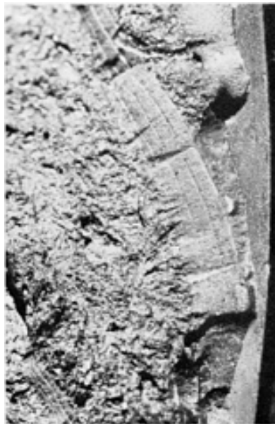
Fig. 452 View of an area at arrow D in Fig. 451, in the region of final fast fracture. Fatigue patches are interspersed among areas of rapid crack advance, indicating that final fracture occurred in stages. 10x
