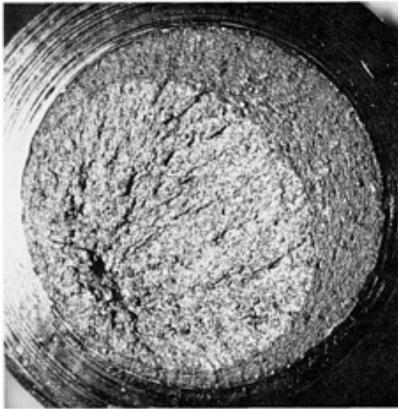
Fig. 430 Surface of a tension-overload fracture in a notched specimen of AISI 4340 steel the same as the specimen shown in Fig. 429, but tested at 80^{\circ}\text{C} ( -110^{\circ}\text{F} ). A fibrous zone, which originated at the notch, surrounds a radial zone, which is off-center because of nonsymmetrical crack propagation. 17\times
