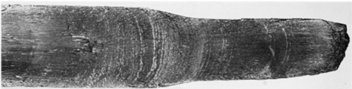
Fig. 206 Mating fracture surface to the one shown in Fig. 205. This piece of the shaft broke away during service. It is believed that the crack propagated a long distance in the longitudinal direction because of weaknesses associated with the presence of longitudinal bands of elongated manganese sulfide inclusions. ~0.5x
