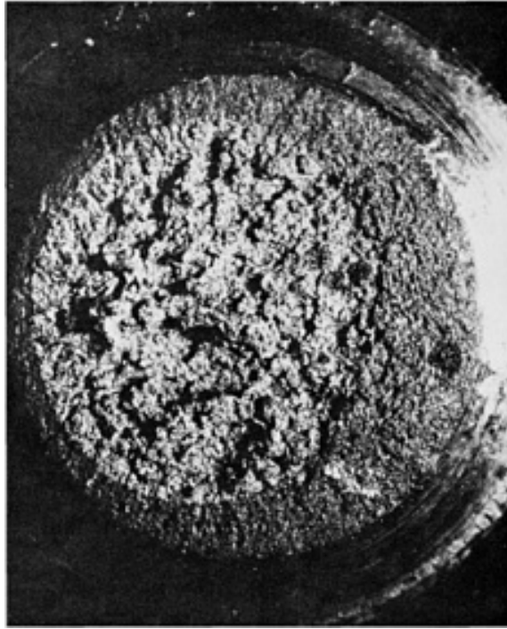
Fig. 427 Surface of a tension-overload fracture in another notched specimen of AISI 4340 steel, the same as in Fig. 426, but tested at -120\text{ }^{\circ}\text{C} ( -185\text{ }^{\circ}\text{F} ). Two distinctly different fracture-surface zones are visible; a fibrous zone, which originated at the notch, surrounds a radial region of final fast fracture. 17\times
