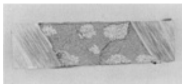
Fig. 80 Example of the macroscopic appearance of hydrogen flakes in plate steel. 1.6 ×
