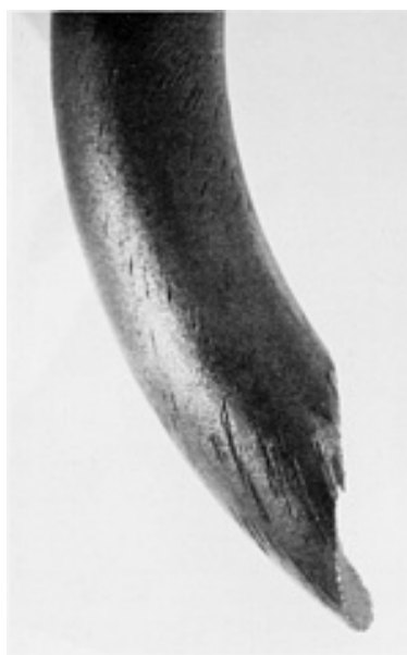
Fig. 265 Fractured 13-mm ( \frac{1}{2} -in.) diam spring of AISI 10B62 steel wire with a hardness of 477 HB. Note the spiral gouges, which are screw marks that were generated during coiling. See also Fig. 266. 2×
