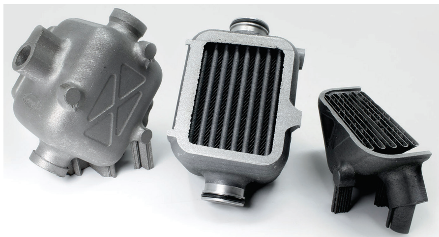
Fig. 3 — A variety of 3D-printed heat exchanger components (both whole and in cross section) demonstrate the design freedom provided by advanced AM technology. Note the ultrathin features in the core (cross section image). Such complexity is nearly impossible to attain with existing AM technologies.
