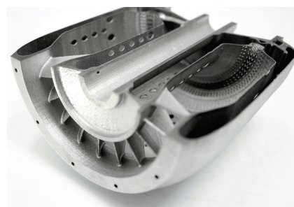
Fig. 4 — Unicore of a 20-kW microturbine engine, being developed by Sierra Turbines, 3D printed on an advanced metal AM system. The nickel-base alloy is exceptionally resistant to stress corrosion cracking and oxidation and is most often used to manufacture parts for combustion-zone gas turbine engines due to its high temperature strength.
