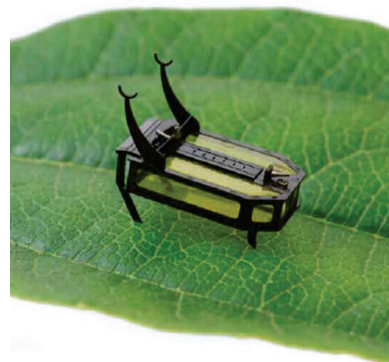
Look ma, no wires! A tiny robotic beetle crawls, carries, and climbs without being connected to a power source. Courtesy of X. Yang, et al./Sci. Robot.
