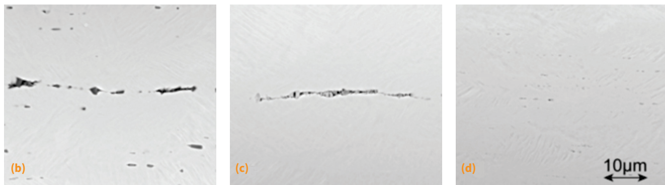
Fig. 2 — (a) Probability of Nitinol diamond fracture at 10 million cycles versus strain amplitude plots for Generation II VAR, Generation II VIM/VAR and Generation III VAR/EBR. (b) Generation II VIM/VAR microstructure showing a ~40 \mu\text{m} long oxide inclusion along with a mixture of smaller oxide and carbide particles. (c) Generation II VAR microstructure showing a ~40 \mu\text{m} long oxide inclusion "stringer" with voids. (d) Generation III VAR/EBR microstructure showing a dispersion of \leq 5 \mu\text{m} oxide inclusions. After Pelton et al. [9] .
