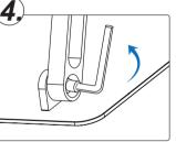
If the friction of hinge is too strong or too little for adjustment, you can use the wrench to adjust.
