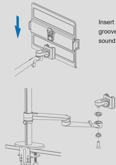
Insert the Laptop Plate into the groove, when heard a click sound means done.
