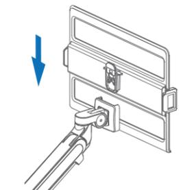
Insert the Laptop Plate into the groove, when heard a click sound means done.
