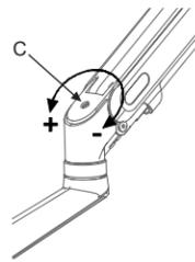
**ADJUST SPRING ARM AT VERTICAL DIRECTION**
