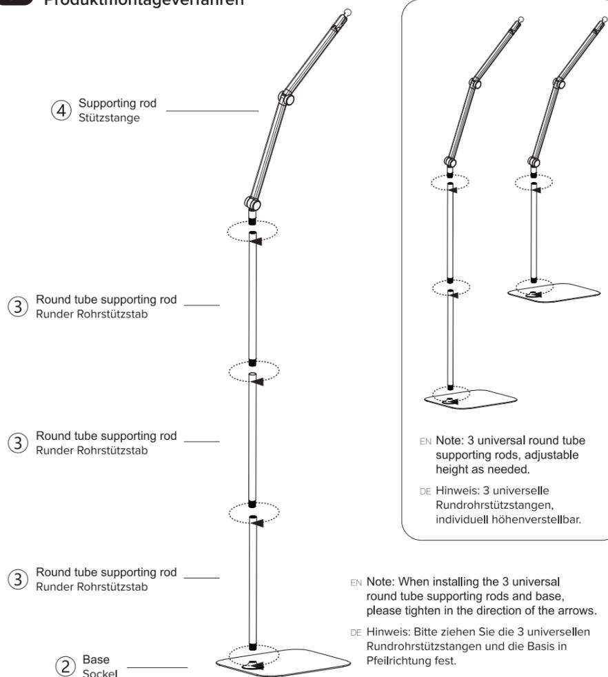
EN Note: 3 universal round tube supporting rods, adjustable height as needed.
