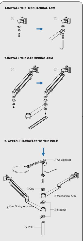
Install the hardware to the pole in sequence as shown.
