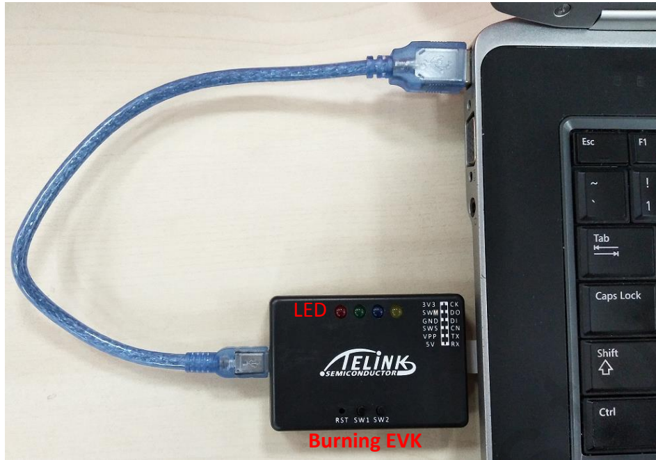
Figure 3 Connect burning EVK with PC
