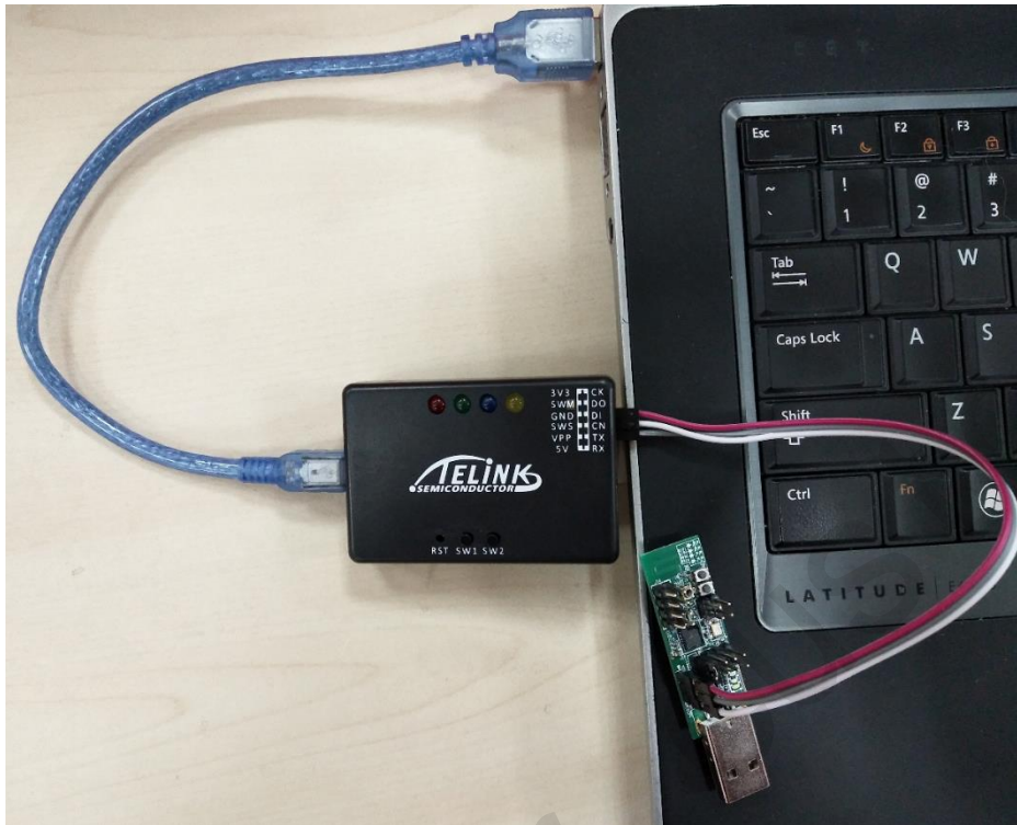
Figure 5 Connect target board with burning EVK via Swire
