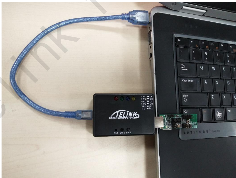
Figure 4 Connect target board with burning EVK via USB
