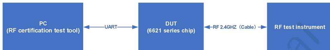
Figure 2.1 Instrument Connection Diagram
