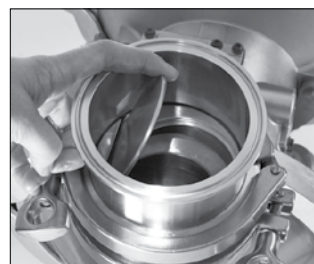
Flapper Check Valve
