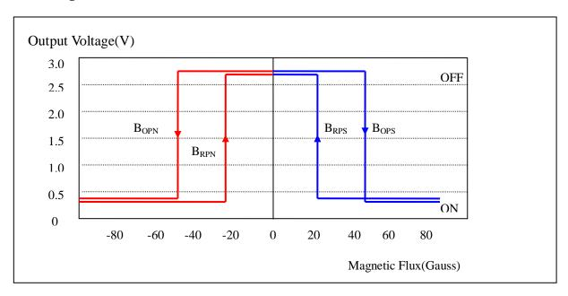
Operating Parameters:  $T_A = 25$ °C,  $V_{DD}=2.75V_{DC}$ .
