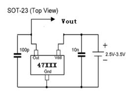
It is strongly recommended that an external bypass capacitor be connected (in close proximity to the Hall sensor) between the supply and ground of the device to reduce both external noise and noise generated by the chopper-stabilization technique. This is especially true due to the relatively high impedance of battery supplies.
