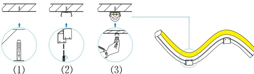
Bending neon strip correctly, fix clip on the surface of application, 2pcs/m, and fix one more clip on turning place
