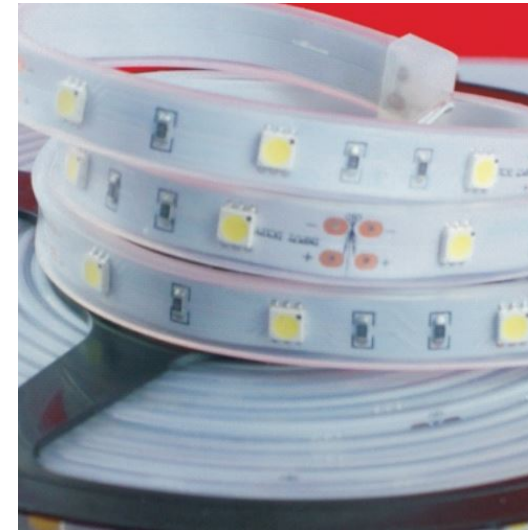
Waterproof A (IP54): Full silicone tube
