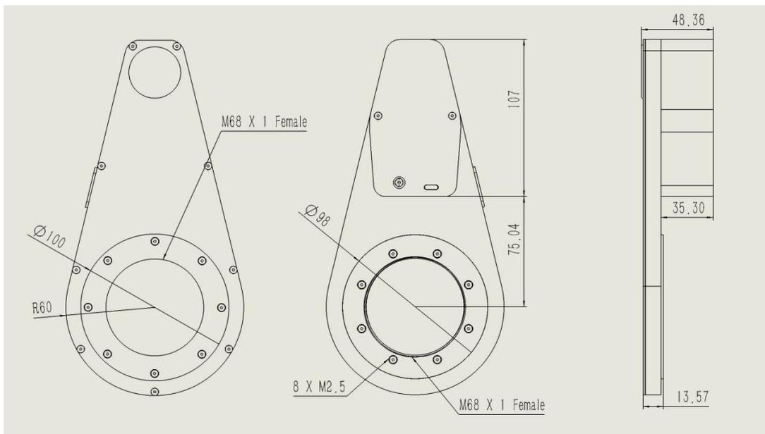
Figure 1 Dimension of WandererRotator Lite
