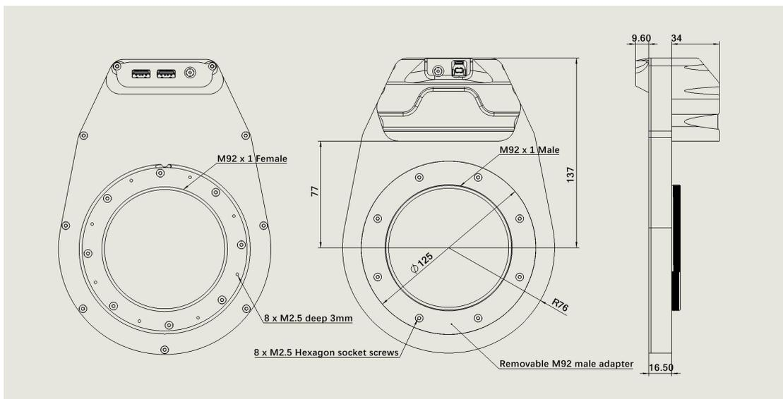
Figure 1 Dimension of WandererRotator Pro
