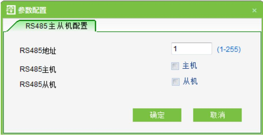
The screenshot shows a software window titled "参数配置" (Parameter Configuration) with a sub-tab "RS485主从机配置" (RS485 Master/Slave Configuration). The window contains the following elements:
