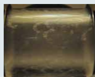
80% dryness fraction ( x = 0.8 ) 20% condensate (with annular flow) → Alarm ⚠
