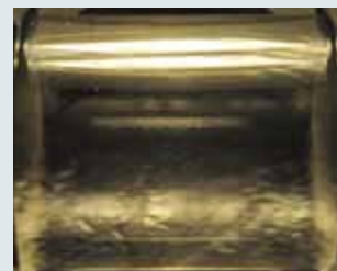
90% dryness fraction ( x = 0.9 ) 10% condensate (with wavy flow)
